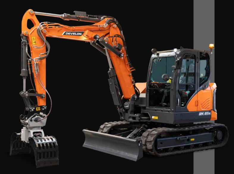
Maximum power48.5 kWOperating weight9528 kgBucket capacity0.28 m³
