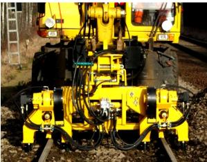
Quick connecting elements at the attachment ensure the simple and safe connection to the excavator's boom and hydraulic system.
